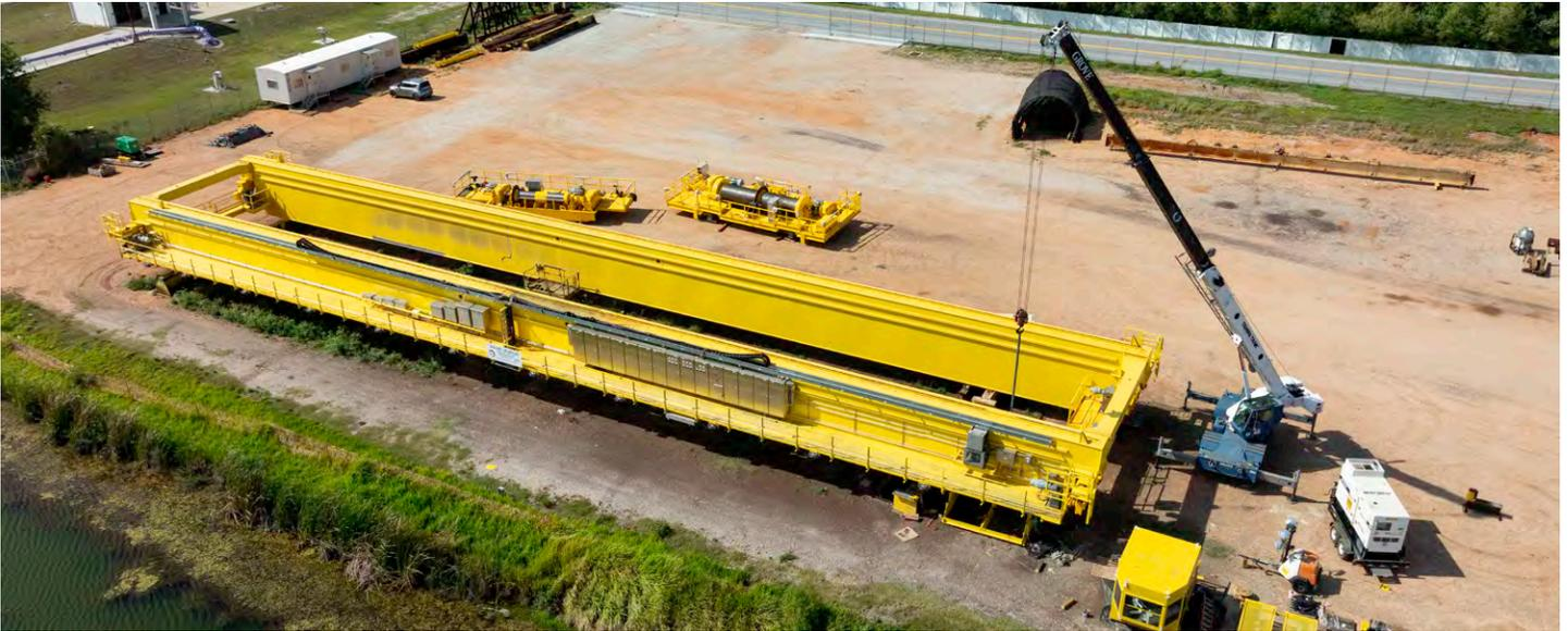
PB has successfully completed fabrication, assembly, and coatings on two massive overhead crane systems for a valued customer. These cranes were custom-made to meet the highest standards of quality, safety and performance based on our customer's design. They measure 12' in height, 30' in width, 195' in length, and can lift up to 120 tons each. The cranes are designed to handle heavy-duty industrial
