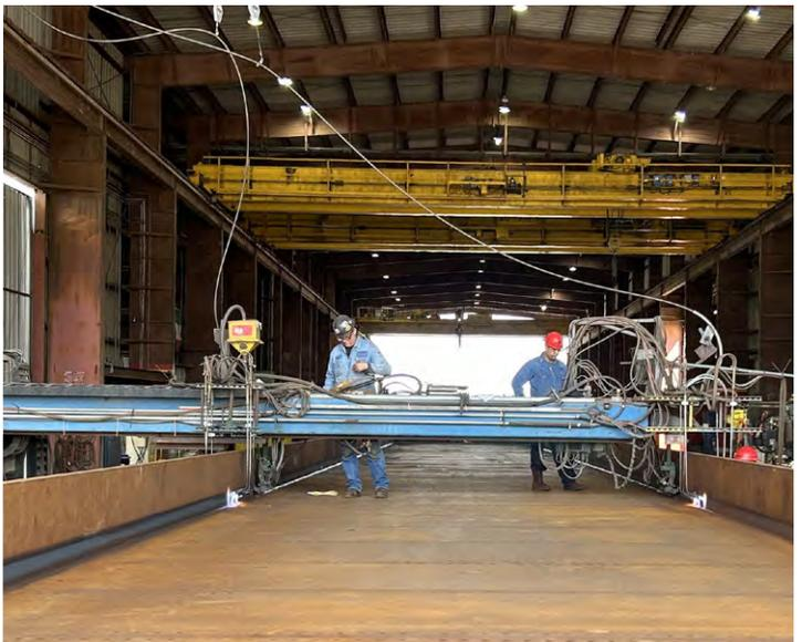
We are proud to announce that our PB team is nearing completion of a massive railroad bridge project for a client in the Northeast U.S. This bridge consists of two main girders that are 150' long, 14' 6" tall, and weigh 275,000 pounds each. The girders for the two structures have web plates that are 1.5 inches thick and flange plates that are 3
